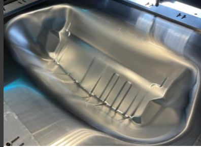
Automotive Interior 6061 – O Aluminum 36" x 48" x 0.063" 46 minutes
