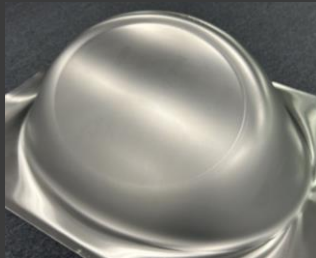
Deep Aluminum Part 6061 – O Aluminum 36" x 48" x 0.125" 50 minutes
